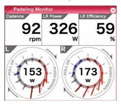
The Force Vector Display gives real-time 12-point pedal stroke analysis on a Pioneer head unit, and can also be viewed post-ride on the Cyclo-Sphere web-based software.
